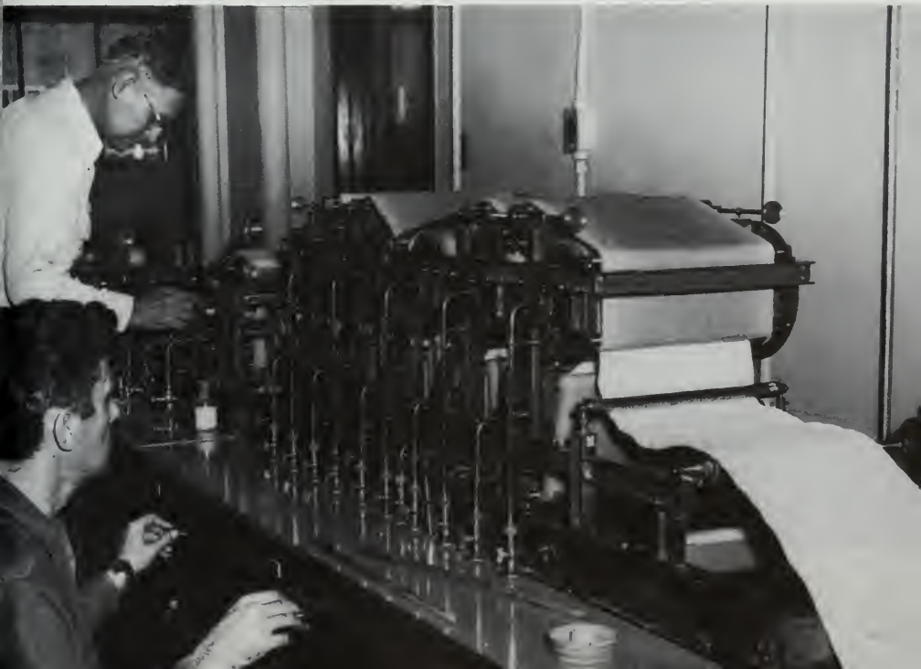
L. E. Talley and D. E. Smith, physical science technicians, use a model of a commercial paper machine to convert experimental pulps to paper.
